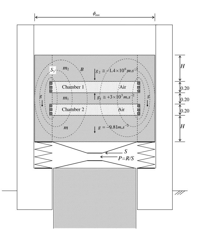
Fig. 15 – Gravitational Press
