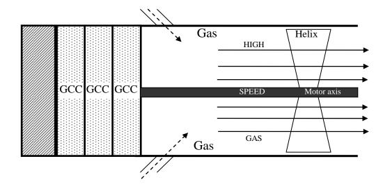
Fig. 12 - The Gravitational Turbo Motor - The gravitationally accelerated gas, by means of the GCCs, propels the helix which movies the motor axis.
