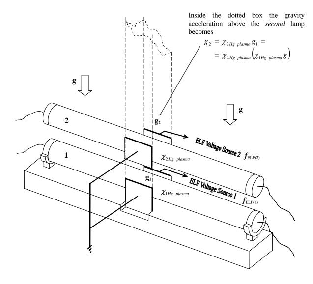
Fig. 2 – Gravity acceleration above a second fluorescent lamp.
