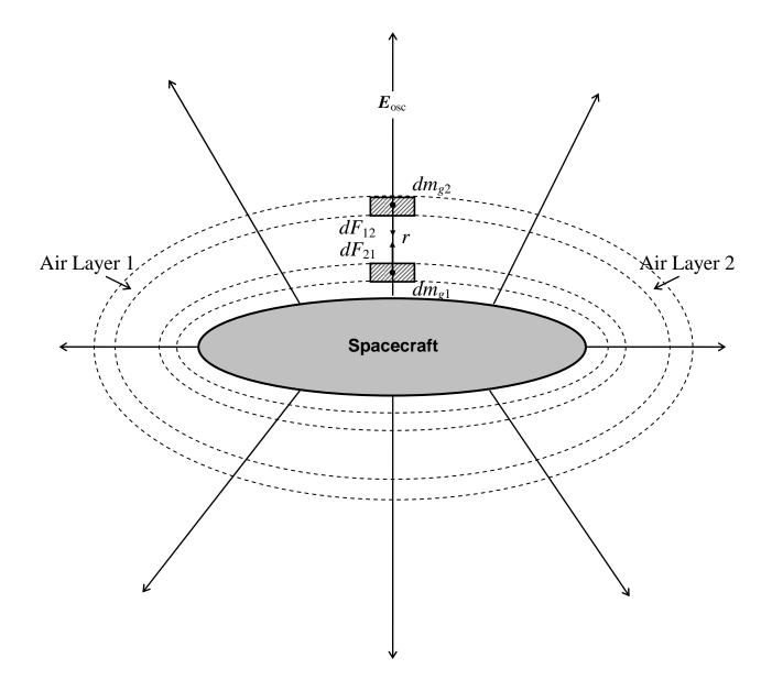
Fig. 13 – Gravitational forces between two layers of the "air shell". The electric field  $E_{osc}$  provides the *ionization* of the air.
