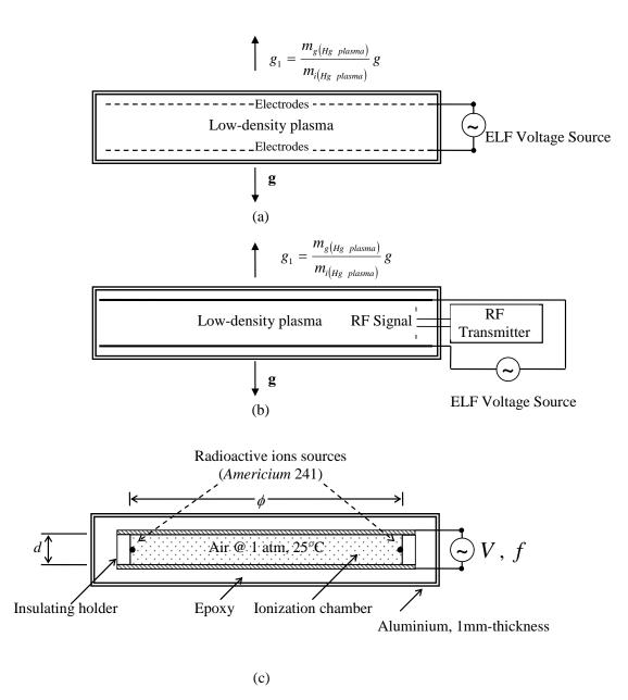
Fig. 3 – Schematic diagram of Gravity Control Cells (GCCs).
