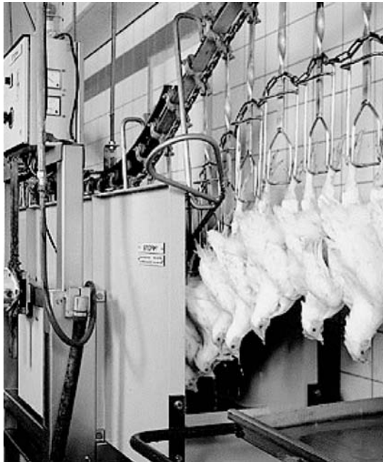
FIGURE 6 Shackled live birds being moved to the point where they will be submerged in an electrical water bath stunner.
