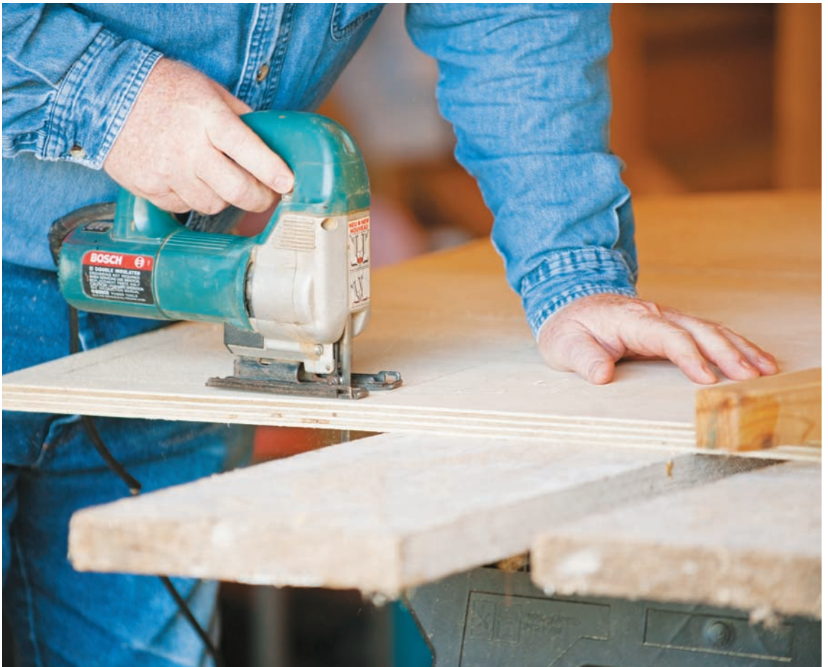
A jigsaw can make the job of cutting the removable coop wall door very simple.
