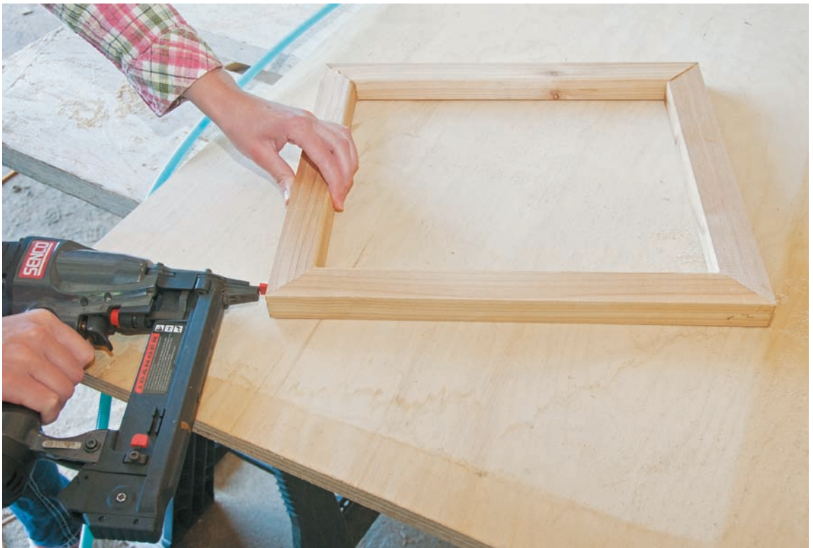
Narrow pieces of wood can easily split accidentally when they're being nailed, so take care. When used safely, an air nailer can be very good for handling this task.
