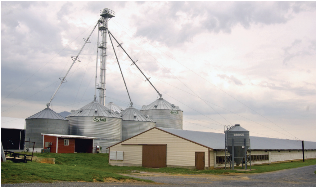
Figure 9.1 A system for storing and delivering feed for poultry. (Courtesy USDA NCRS; photograph by Bob Nichols.)
