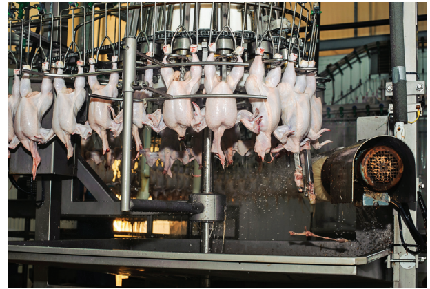
Figure 19.7 Chickens in shackles on the line in a poultry processing plant. (Source: Sergey Bogdanov/ Shutterstock)
