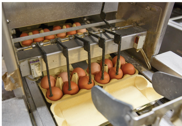
Figure 18.22 Automated packaging of chicken eggs in an egg packing facility. (Source: zlikovec/Shutterstock)
