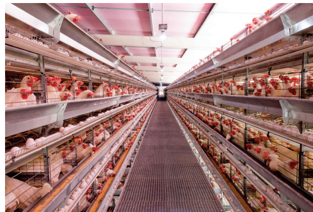
Figure 18.12 Conventional cages for hens in a layer house. (Courtesy of Big Dutchman)
