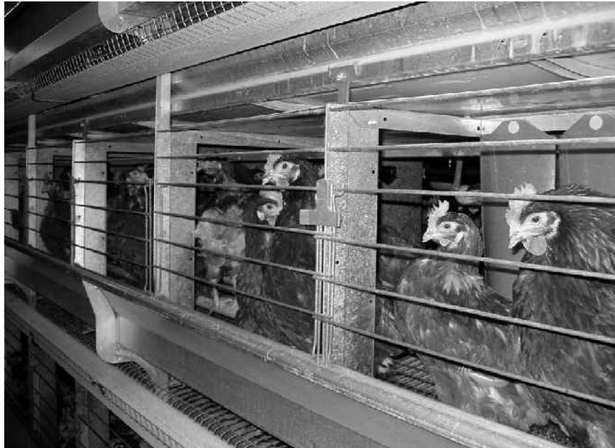
Fig. 11.4. German-made large furnished cage (FCL) with 60 hens. Similar design to that shown in Fig. 11.3 but without centre feed trough. Overall size 362 cm wide × 125 cm deep approximately.
