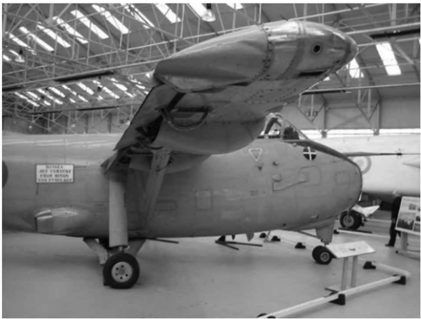
FIGURE 3.34 The H.126's blown flaps with wing tip thrusters and main exhausts. (After: Mark.murphy [64].)
