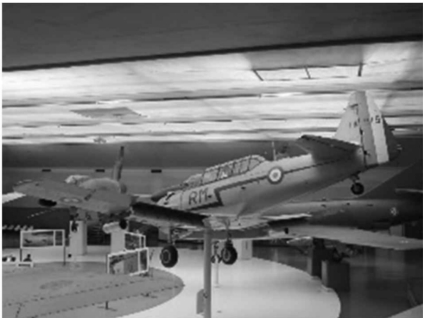
FIGURE 3.21 North American T-6 trainer showing its split flaps. (After: 2009 [18].)
