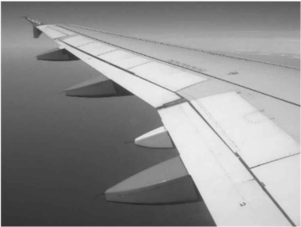
FIGURE 3.22 The three orange pods are fairings streamlining the flap track mechanisms. The flaps (two on each side, on the Airbus 319) lie directly above these. (After: [19].)
