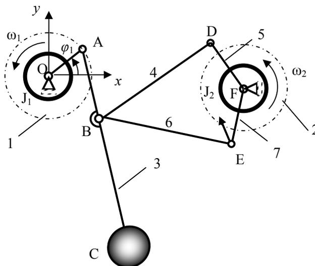
Figure 1. Typical graphical representation of G. Constantinescu torque converter mechanism
