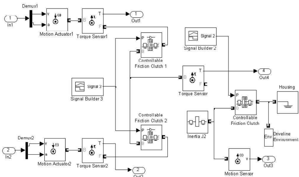
Figure 3. The Simulink model of unidirectional mechanism
