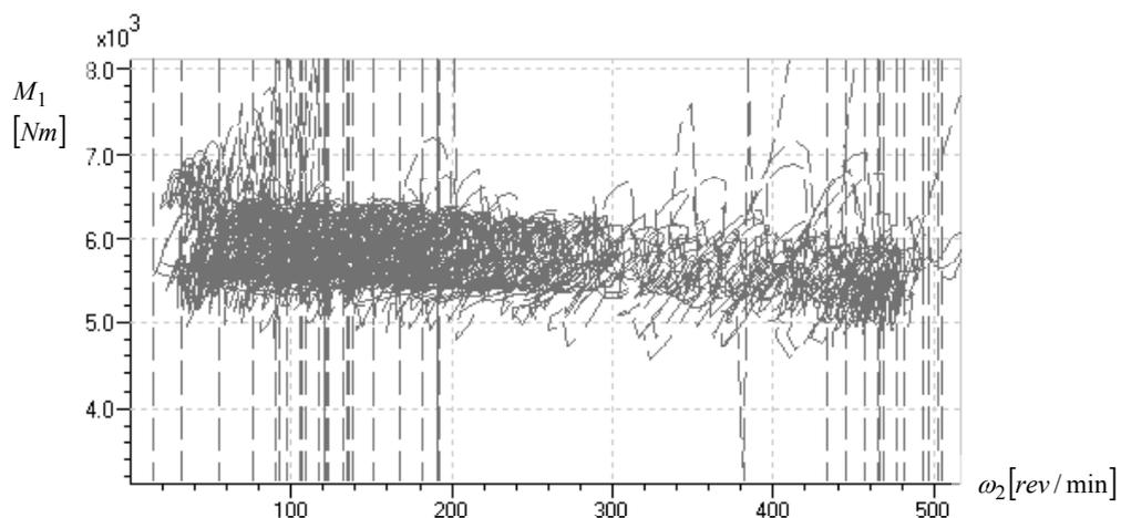
Figure 6. Input torque diagram  $M_1(\omega_2)$
