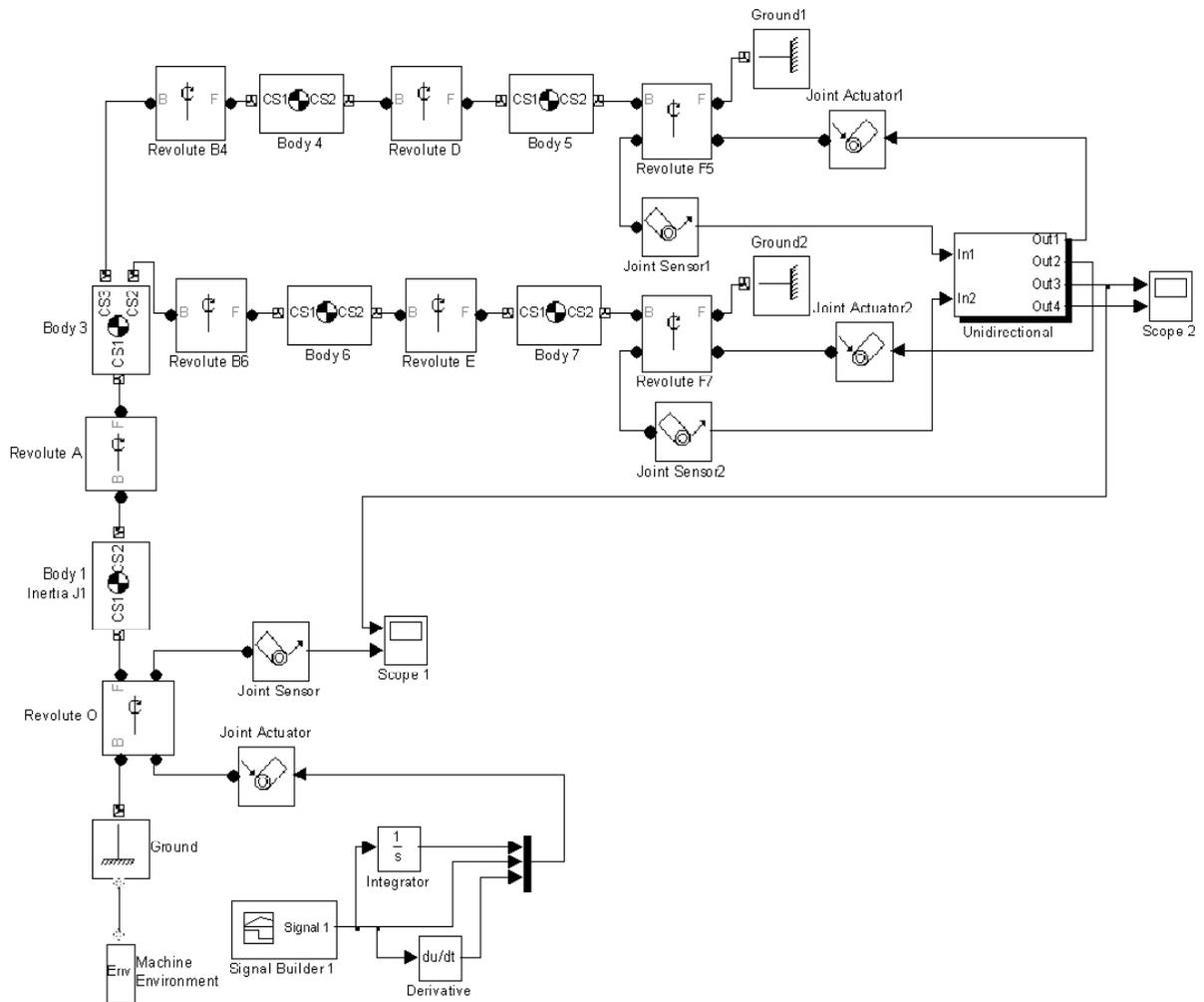
Figure 2. The Simulink model of torque converter mechanism
