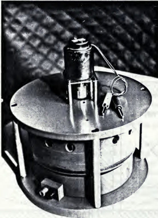
Fig. 18. - The second VENETIN COLIU machine constructed by Marinov in February 1991. The d.c. motor on the top drives the rotor.
