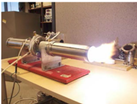
Operational 10 kW Gliding Arc Plasmatron
