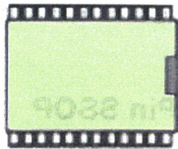
14-Pin SSOP Area = 48 mm 2
