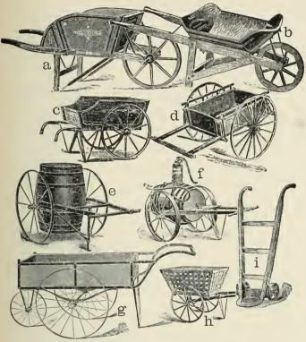
Fig. 31. Various barrows, carts and trucks. All of which are useful for the gardener. *f* is a good type of hand spray pump for small areas.
