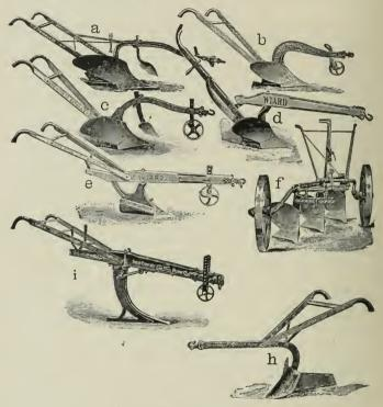
Fig. 26. Various types of plows. f is a gaug-plow, turning three furrows at once; h is a winged shovel or furrowing or hilling plow; e and i are subsoil plows.
