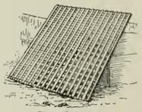
Fig. 36. Lath screen. The spaces and laths are equal in width.
