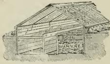
Fig. 16. Manure-heated forcing-house.
