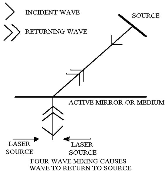
Phase conjugate mechanism or mirror in the laboratory.
