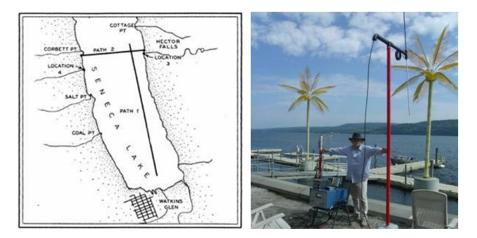
Photo 3. Propagation paths on Seneca Lake used by Burrows in 1936. In 2014 Corum used path 1. The photo shows the Zenneck probe (the small golden doublet, left side) mounted at six feet, and the conventional 52 MHz vertical  $\lambda/2$  dipole with a Guanella balun mounted at 10 feet (right side). Our 2014 data is shown in Figure 4, above. The Texzon technology described herein is Patent Pending.
