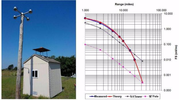
Photo 2. The 4.9 meter 1.82 MHz surface wave probe and field strength measurements (out to 20 miles) compared with predicted fields for Zenneck, a  $\lambda/4$  tower (with 120 radials), and the actual Norton vertical stub with only an 8 ft. ground rod at the base of the pole. [2/12/2016: C = 45 pF, V<sub>RMS</sub> = 42.4 volts,  $\epsilon_r = 15$ ,  $\sigma = 0.012$ ,  $R_g = 35 \Omega$ . For radiation:  $h/\lambda = 0.030$ ,  $R_r = 1.38 \Omega$ ,  $\eta_r = 3.8\%$ .]
