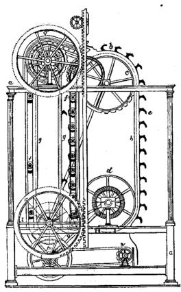
manner:—On the axis  $c^1$  is affixed a bevilled toothed wheel  $c^3$ , which takes into and drives the bevilled toothed wheel k
