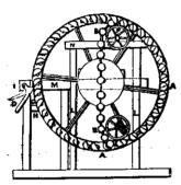
tied together by means of chains, ropes, or straps. This set of weights, forming an endless chain, runs over two pulleys, or rollers, suitably disposed up and down near the fly wheel, which is provided with a set of cups suitably shaped, and fixed around near its periphery, so as to receive the weights as they are delivered up by the upper pulley, and to carry them down to the
