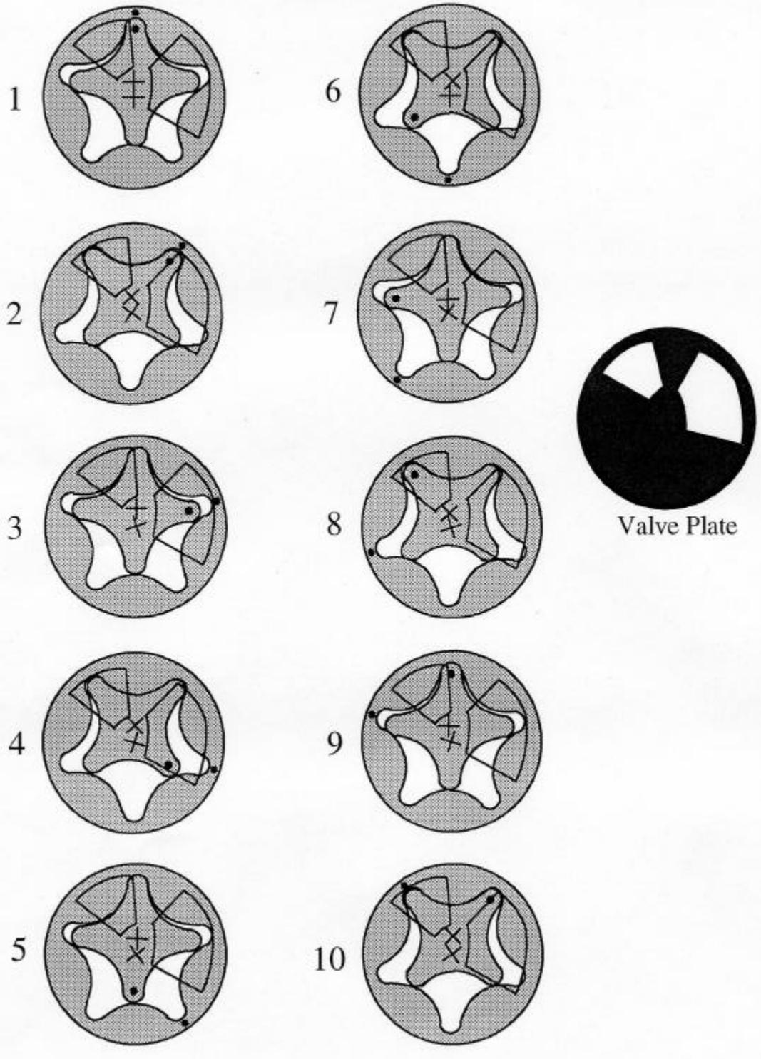
**Figure 2.** Porting for StarRotor compressor.
