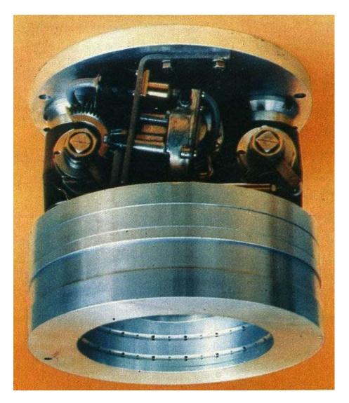
OTRAG injection head in the first phase of the project until 1972, there were already 200 firing tests with 3 failures. By the end of the support by the BMFT, in 1974 there were 2,000 tests and now it will be 6000, with an accumulated operating time of 1 million seconds. I have received from Lutz Kayser no slice of the engine, fearing that someone might steal his intellectual property. The pictures here show, therefore, only the schematic operation.
