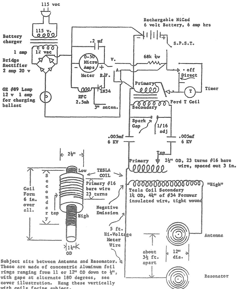
Subject sits between Antenna and Resonator. These are made of concentric Aluminum foil rings ranging from 11 or 12" OD down to 1/2", with gaps at alternate 180 degrees, see cover illustration. Hang these vertically with coils facing subject.
