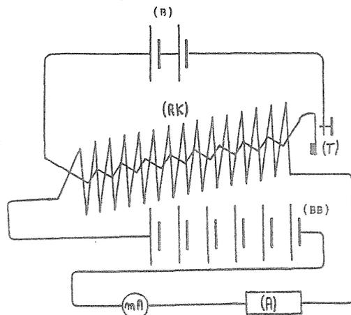
The best way to generate a Faradic current was to employ a Leclanche battery and a Rumkorff coil connected to the electrodes of Figure VI, but the electrotherapists saw it better to combine the two kinds of treatment into the galvano-faradic apparatus of Figure VII where (B) is the battery that feeds the Rumkorff Coil (RK), (T) a make-and-break device, (BB) the Leclanche battery-grouping for galvanic treatment, (mA) a milliammeter and (A) the patient to be treated.
