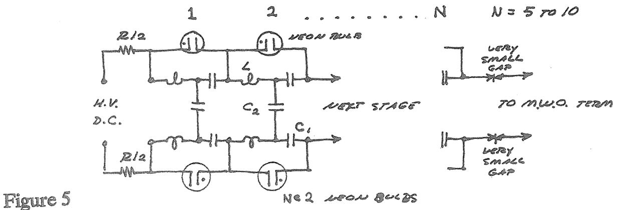
D.C. INPUT = 240V / STAGE ALL C<sub>1</sub> RATED 600V
