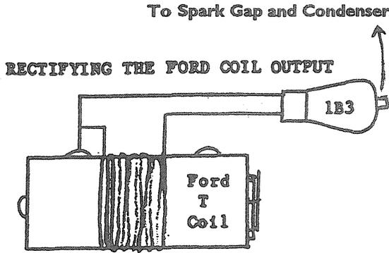
Wind 15 or more turns of fairly heavy insulated copper wire around the middle of the Model T Ford Coil. One lead from the winding goes to the Hi-voltage output of the Coil, and to pin 2 or 7 of the 1B3 tube. The other lead goes to the other pin, as only two pins of the tube, 2 and 7, are used in this hookup. The souped-up or rectified voltage is drawn off the top of the tube to the spark gap and condenser.
