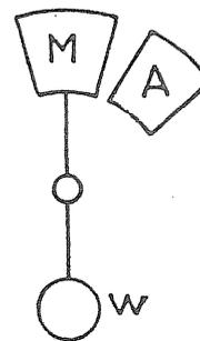
The simplified diagram of the radio-cellular-oscillator is indicated in Figure 9 (Mesny set-up).
