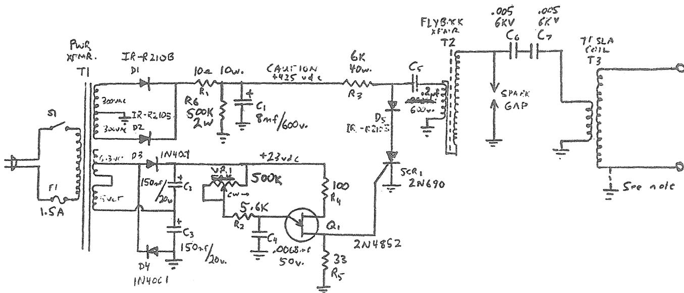
Note: Optional ground for Tesla coil secondary, if it reduces output do not use. R3 made from four 25K 10w resistors in parallel. VR1 linear taper. C1 may or may not be polarized. C6, C7 could be single .0025/15KV capacitor. SCR1, Q1 and all diodes can be standard replacement equivalents. MFR Type: T1 - TRIAD. T2 - Stancor H0 6246, Thordarson fly. Alternate values: R3 - 1K ohm, 225 watts; C5 - 1 microfarad, 600v.
