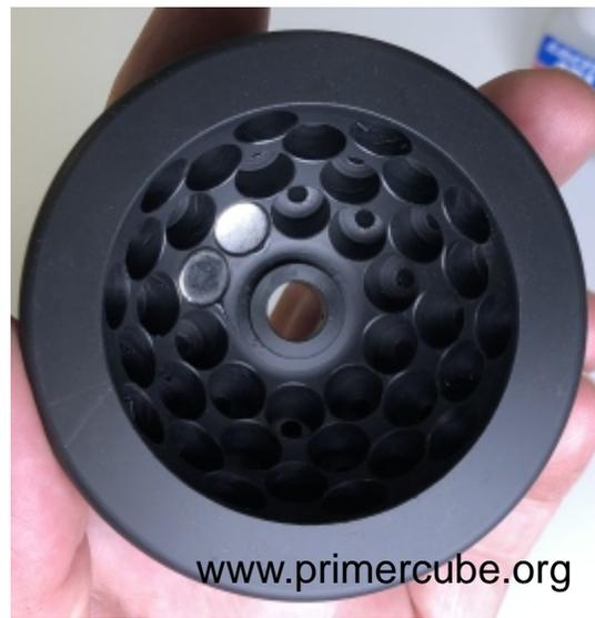
Repeat the process for the second magnet and for each magnet thereafter in the inner ring of magnets. Repeat this process for the second ring, then the third ring and then the fourth ring of magnets until the all 40 magnets are glued in place. This entire process takes about 15 minutes to do by hand but could be done by an automated machine in five minutes or less.
