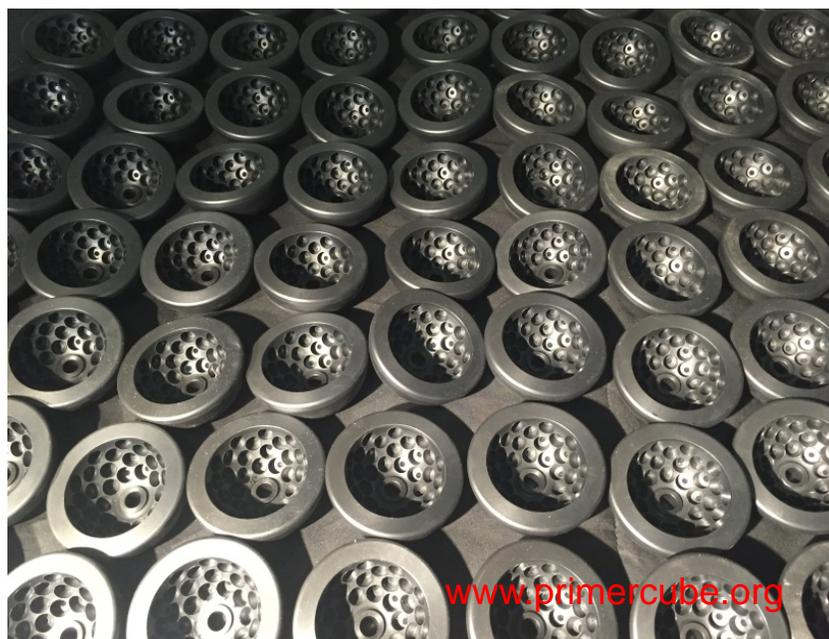
This photo shows a production run of arrays ready for deburring and cleaning to insure good adhesion when gluing the magnets in place. It is also important to inspect each array carefully to insure that no chips remain in a hole which would keep a magnet from being fully seated.
