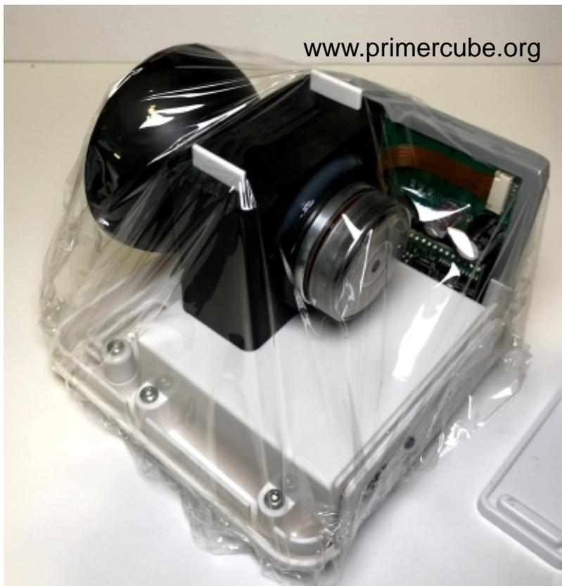
Wrap the entire assembly in plastic wrap to keep shavings and debris from getting into critical parts during the steps to follow.
