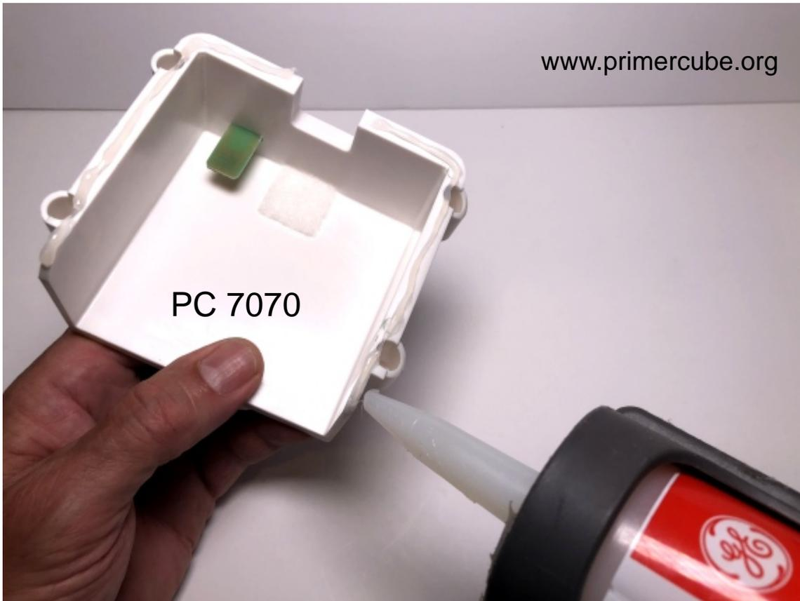
Place a small bead of GE 5100 silicone caulking as shown in photo above.
