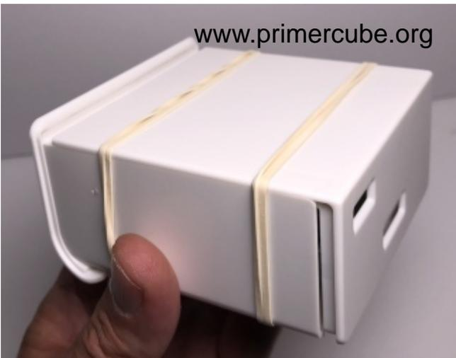
Place PC 7020 into position on PC 7010 as shown and secure with rubber bands. Leave a space for the silicone sealant in the next step.
