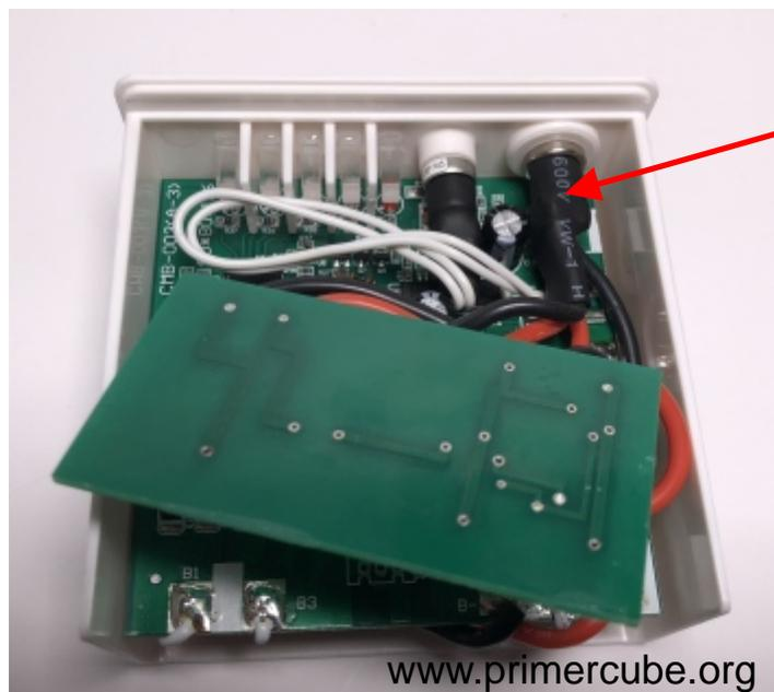
Place the input socket into the proper hole and secure with the washer and nut.
