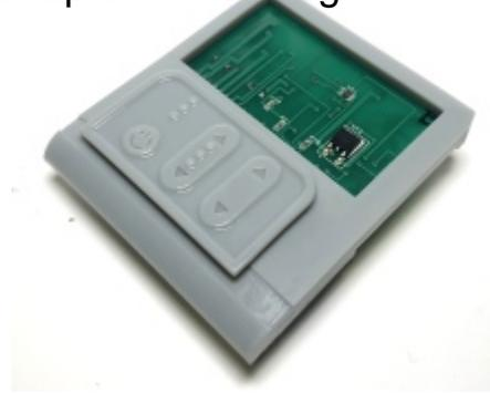
Insert PrimerCube Motherboard into PC 7200 and then place into PC 7000 as shown below.
