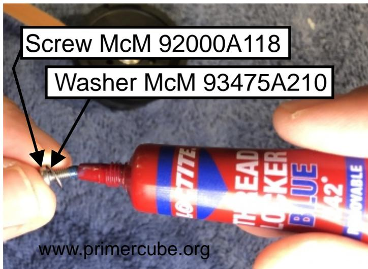
Place the washer onto the screw and then apply a small drop of threadlocker onto Screw McM 92000A118. Be careful that no excess threadlocker can drip off of the screw and into the motor as that could lead to undesirable problems.
