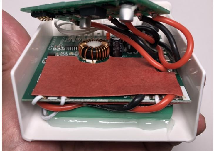
Place self adhesive insulating paper over the area of the lower PCB shown above.
