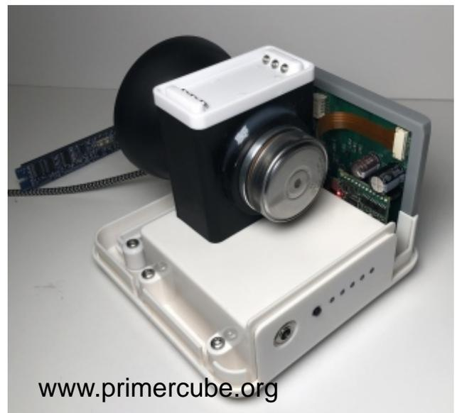
Insert a charged battery pack into the PrimerCube as shown.
