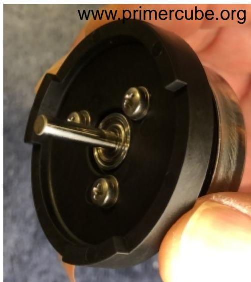
Place the screw into the hole and tighten firmly but do not over tighten. Repeat the process for the other two screws. This photo shows the motor with Part # PC 8700 attached with the three screws.
