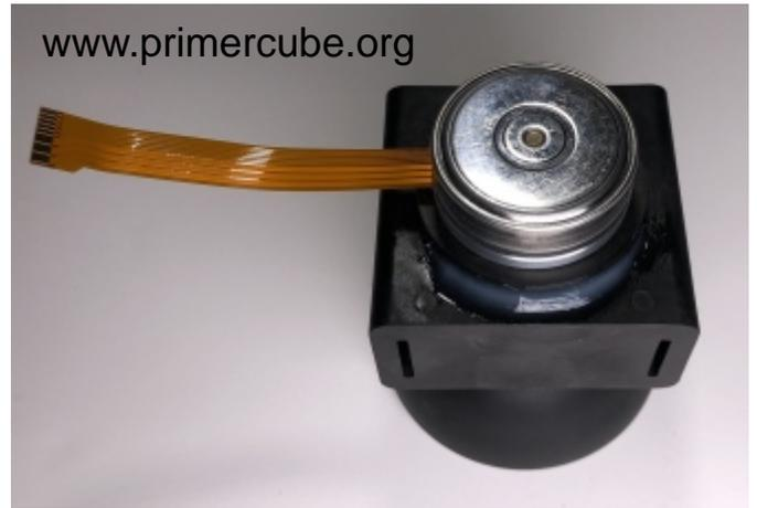
After pressing the Maxon motor into place put a small amount of GE 5100 or equivalent as shown above. Skipping this step can lead to undesirable vibration when the unit is running. Before running this assembly it should then set for 24 hours to allow the curing of the threadlocker, the Loctite 648, and the silicone.
