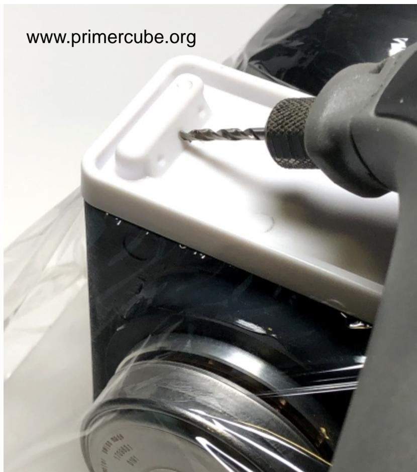
Using a .077 inch diameter drill bit make six holes in the locations indicated by the marks on PC 8600. The holes should be about 1/2 inch deep. Keep the drill bit at 90 degrees to the surface with the location marks as shown in the photo.
