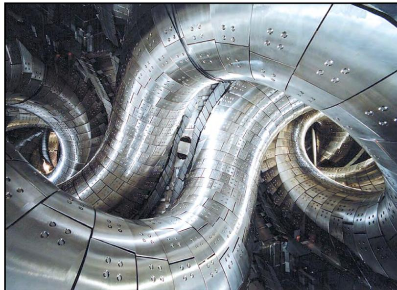
**The Heliotron magnetic field containment device.** The Large Helical Device (LHD) project involves construction of the world's largest superconductor helical device, which employs a heliotron magnetic field originally developed in Japan. The objectives are to conduct fusion-plasma confinement research in a steady-state machine and to elucidate important research issues in physics and engineering for helical plasma reactors.
