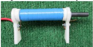
$L_1$ . It must be wound over an open ferrite core as shown in Fig. 7.9. (A coil with a ring ferrite should not be used because of saturation caused by the initial current from the capacitor discharge).
