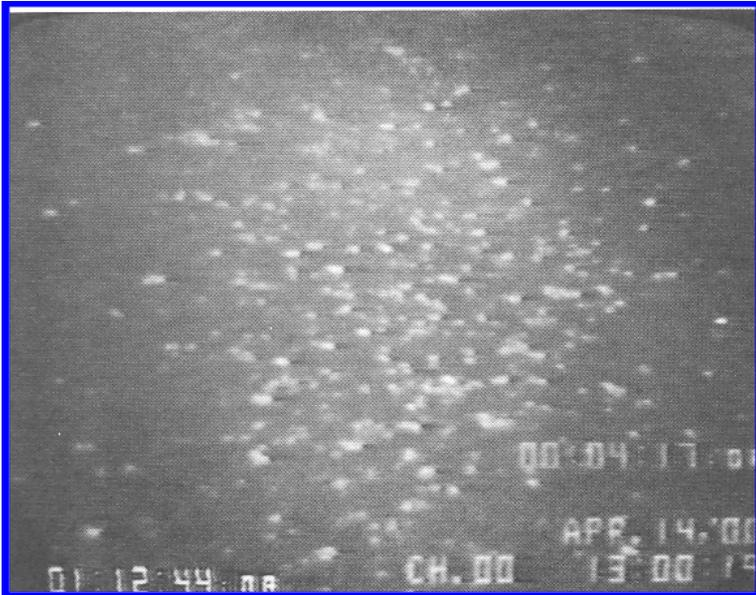
**Fig. 17 Pinhole Camera Image of Particles Ejected From Rear of Aluminum Foil.**
