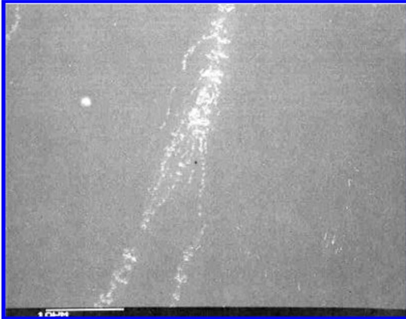
**Fig. 3 SEM of EVO Skipping Across Film of Aluminum on Glass.**
