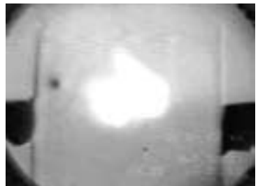
Fig. 12. A higher intensity shot similar to Fig. 11. A test for X rays was run but only a trivial level was found. The image is formed primarily from point source electrons.
