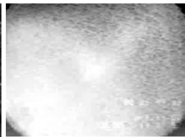
Fig. 6. Saturation level of electron multiplier occurs in most of the field of view. The video camera has also reached saturation. The multiplier was blown out in the next frame.
