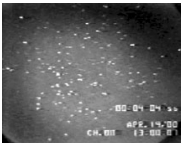
Fig. 2. Light bombardment of a 0.001" thick aluminum target spaced about 1/4" from the imaging pinhole. Specks are clusters of electrons.
