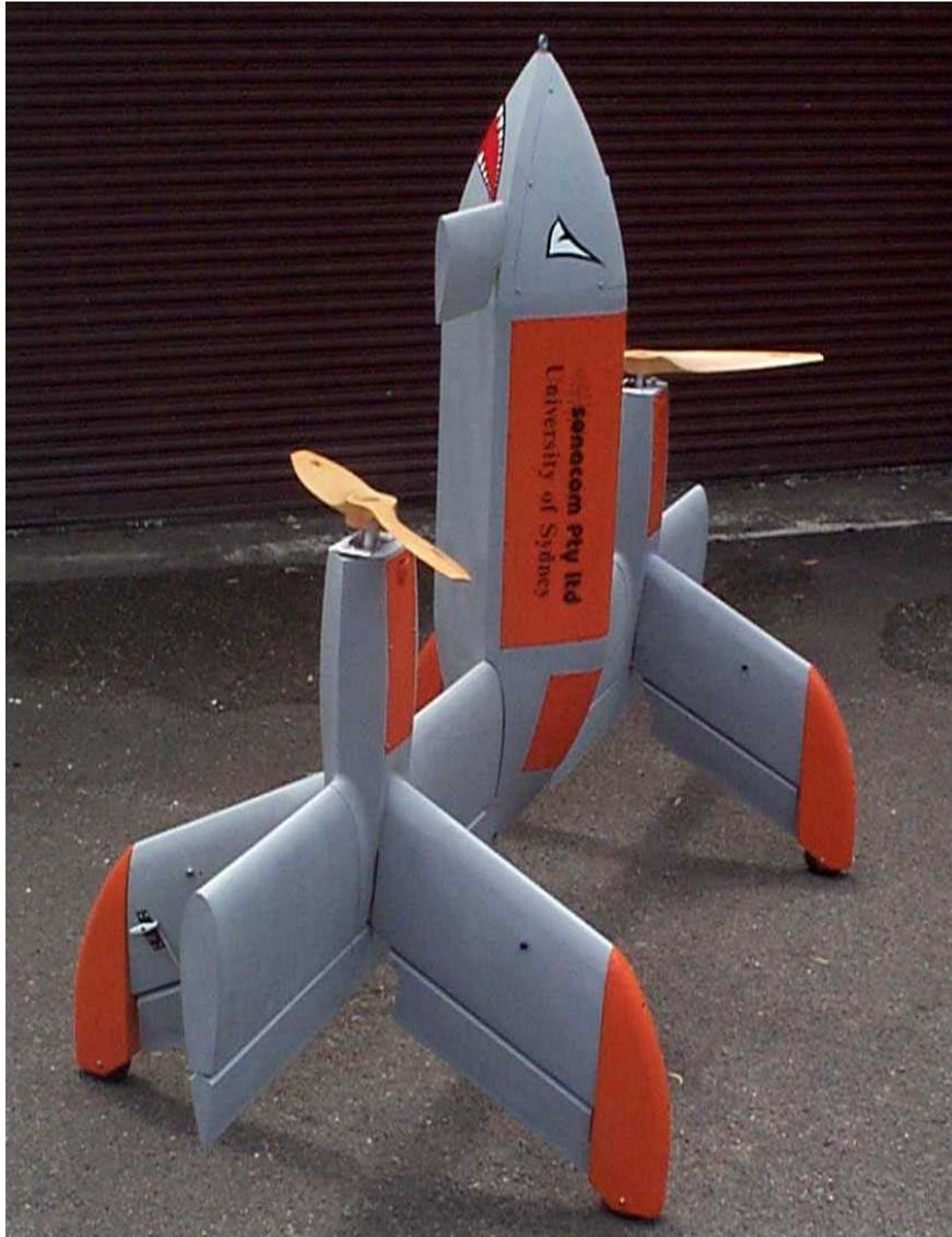
**Figure 6: Completed T-Wing Technology Demonstrator Vehicle, (Electric Powered Configuration).**
