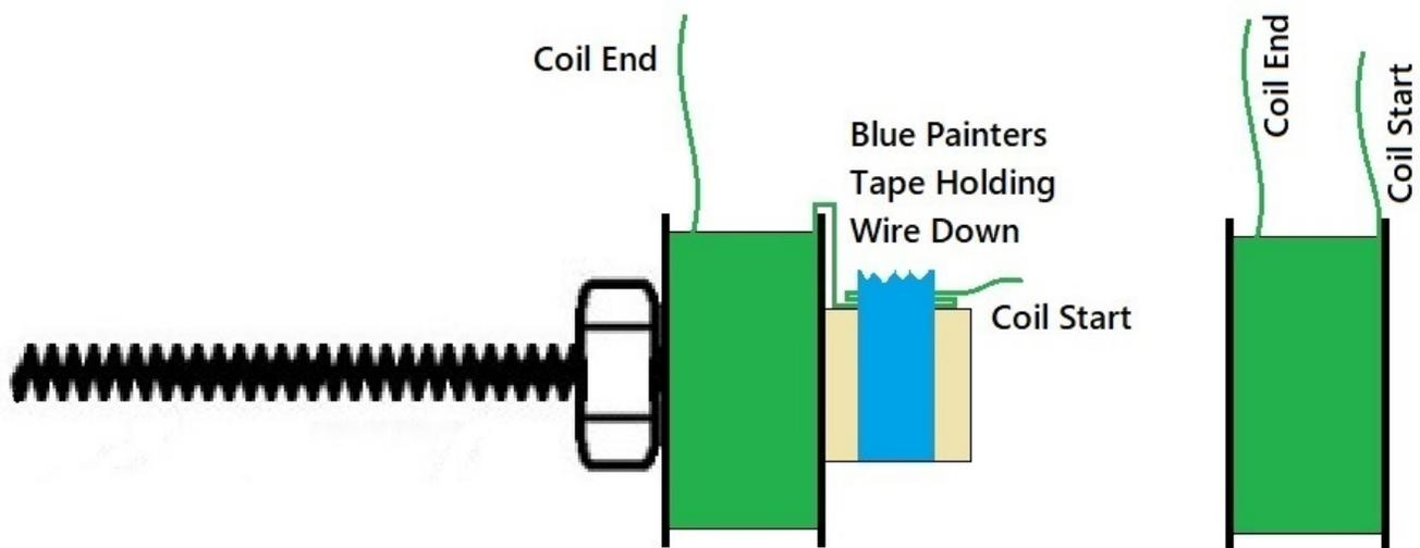
**Hold the wire between the Winder and the Wire Spool with a folded up paper towel, your fingers will thank you for it. Start the drill slowly increase the speed as you get the hang of winding the coils.**
