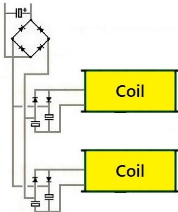
**The Power Recovery Circuit allows energy to be collected from the rising and falling magnetic field of the remaining coils on the rotor.**
