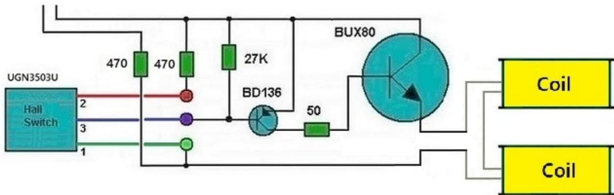
**The Hall Switch is best described as a magnetic lock. A magnetic field coming close to it is the key that opens the lock allowing current to flow. Embed small round bar magnets in the rim of the rotor and mount the hall sensor close to the rotor's rim.**
