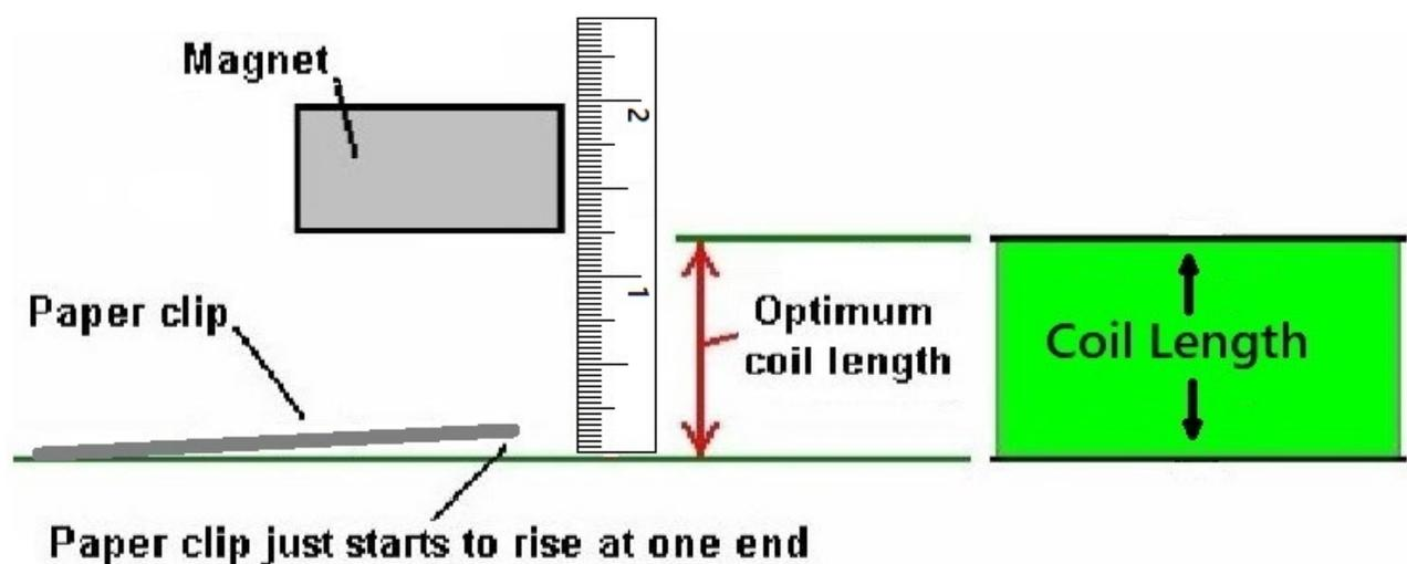
**Hold one of the Rotor Magnets against a wood or plastic ruler over the end of a large paper clip, Slowly lower the Magnet until the paper clip starts to rise off the table. You might have to do this a couple times because the paper clip will jump up to the magnet really fast once it starts to be influenced by the magnetic field.**
