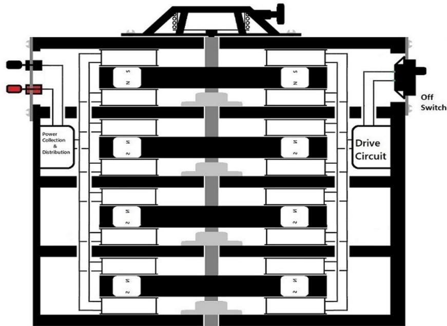
**Creating a larger device can be as simple as making a longer Rotor Shaft and additional Rotor and Coil Panels and installing them in a larger enclosure.**
