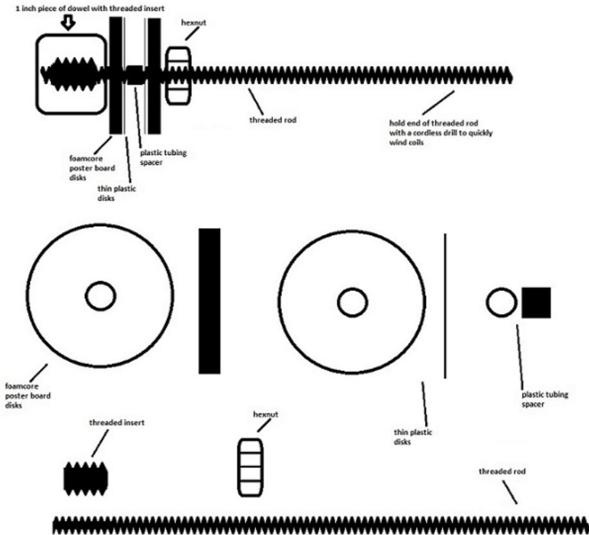
**You'll need to make a simple coil winder like the one depicted above. Clamping the threaded rod in a cordless drill chuck makes it easy to wind coils quickly.**
