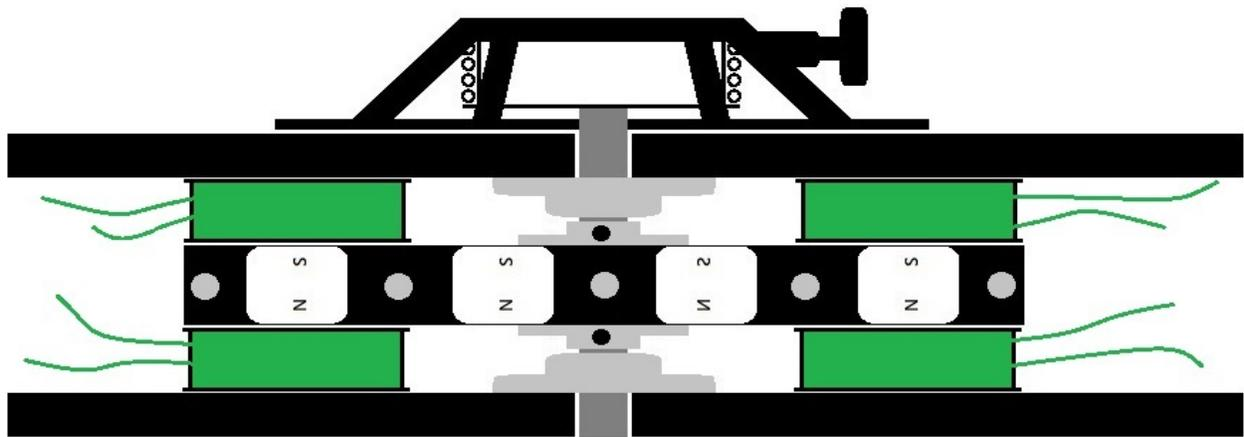
**If you've been making the parts as you go through the manual you should now have the Magnets installed in the Rotor the Coils made and Glued to the square panels and the Rotor Shaft made.**
