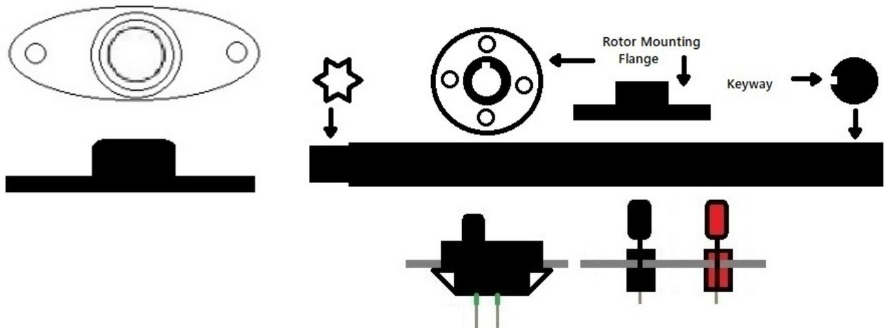
**Bearings, 2 Mounting Flanges for the Rotor to be attached to a Shaft with one end machined to match the Pull Starter Socket.**
