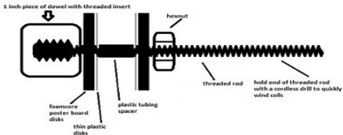
**into the Insert. Slip one Foamcore Disk onto the Rod pushing down to the block of wood followed by one Thin Plastic Disk, one Spacer Tube, another Thin Plastic Disk, another Foamcore Disk and finish by screwing on the Hexnut all the way down to the Coil form. Screw it down**
