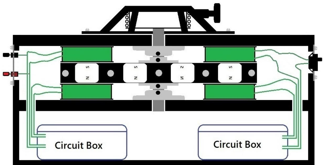
**I can't give you exact measurements for the side and bottom of the box. You'll have to take measurements off the Rotor Assembly. What you're going to do is make three sides and a bottom to be attached to the Rotor**
