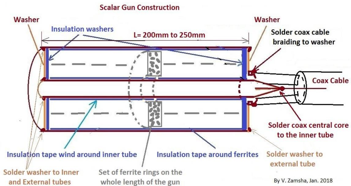
The assembled “head” of scalar gun is connected to the control box via a short coax cable. Control box is a pulse generator with control buttons (not shown here). Average operational frequency of the scalar gun assembled in Belarus by V.Shevstov is around 100kHz, and fed with unipolar square pulses with duty cycle around 10% - on picture:
