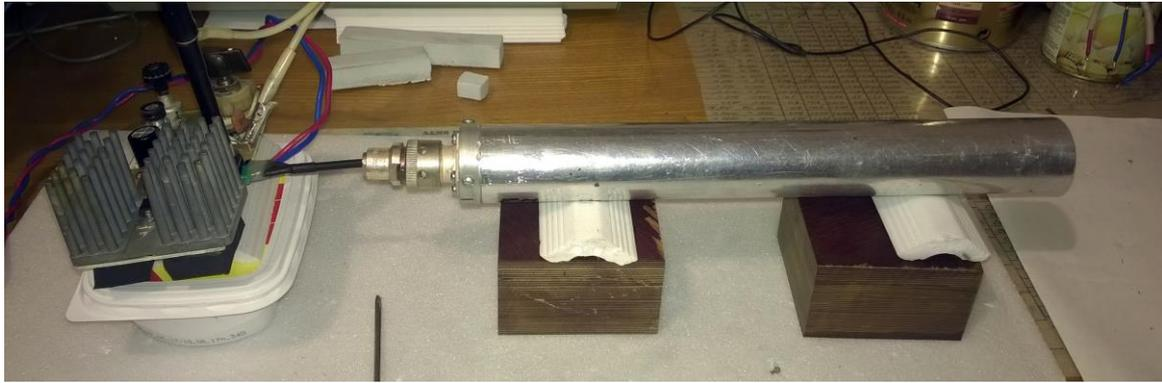
It is assembled from two long aluminum cylinders (outer and inner) and two washers. Internal space between two cylinders filled with toroidal ferrite cores. Sketch of the scalar gun (head) on picture below:
