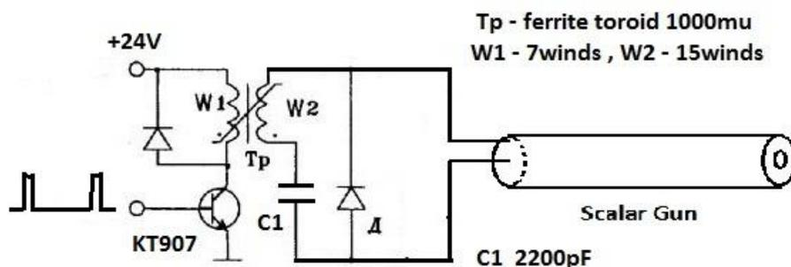
Micro scalar gun consumed around 80mA DC current, amplitude of pulses on inputs of scalar gun was around 33V. Observe phasing of W1 and W2 winds to get correct pulsing!
