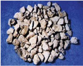
Optical photo of air-cooled slag [80].
