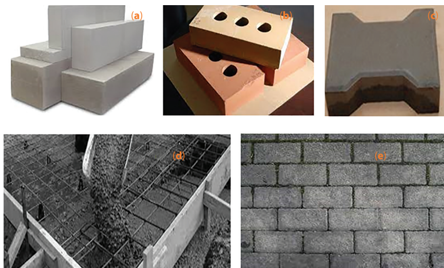
Figure 8.1 Civil engineering geopolymer materials: (a) GP-based bricks, (b) GP-based fired bricks, (c) GP-based paver block, (d) GP-based concrete, and (e) GP-based brick wall.
