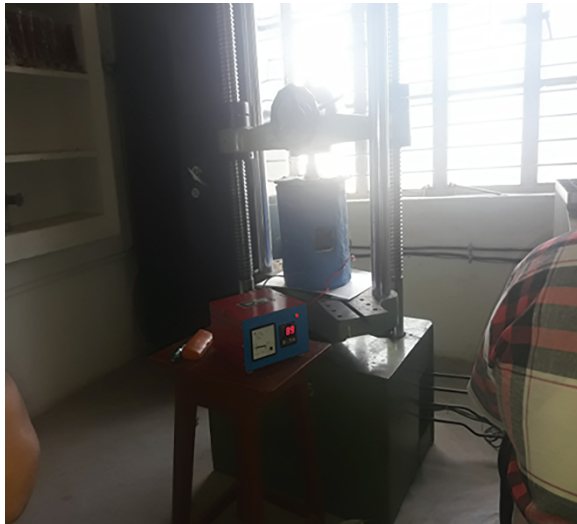
Figure 3.6 MOR set-up (fabricated) for elevated temperature studies.
