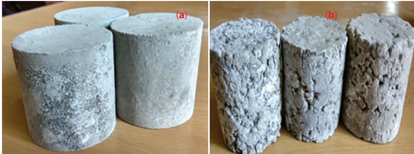
Figure 7.1 Photograph of (a) PA-based geopolymer mortar, and (b) Concrete samples for corrosion study.
