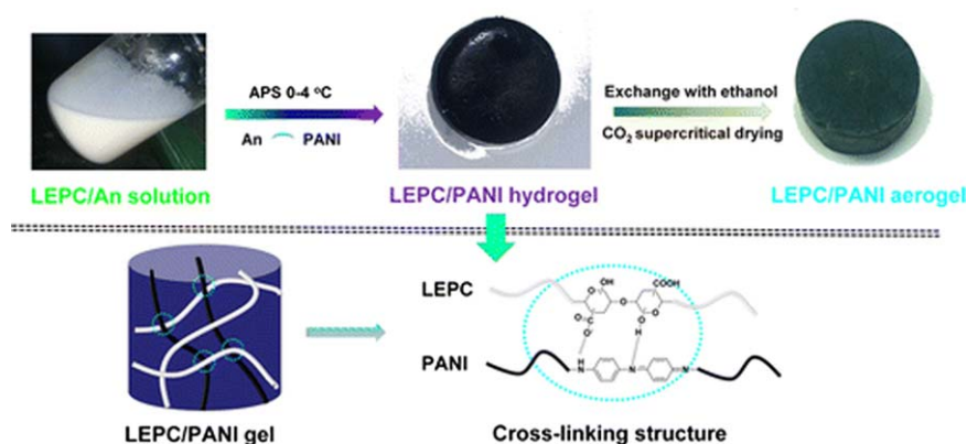
Figure 10.4 Schematic illustration of pectin/PANI aerogel formation. Reprinted with permission from H.-B. Zhao, L. Yuan, Z.-B. Fu, C.-Y. Wang, X. Yang, J.-Y. Zhu, J. Qu, H.-B. Chen and D. A. Schiraldi, ACS Applied Materials & Interfaces , 2016, 8 , 9917–9924, Copyright 2016 American Chemical Society. 20
