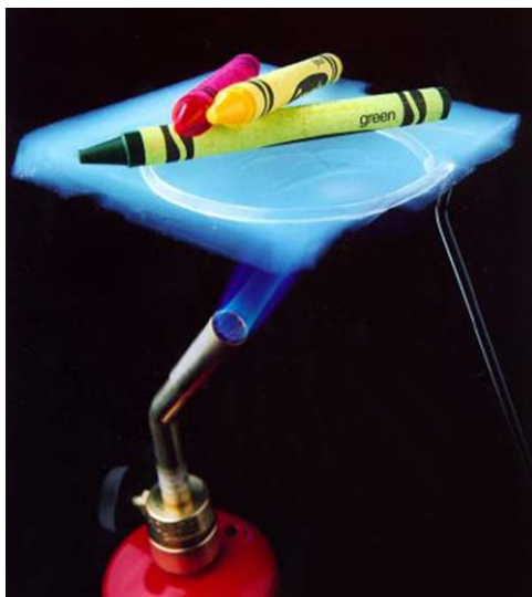
Figure 1.1 The crayons on top of the aerogel are protected from the flame underneath. Reproduced from ref. 1.
