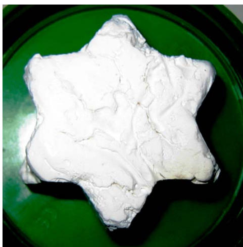
Figure 1.4 Starch aerogel obtained by supercritical drying from a hydrogel prepared in a mould for Christmas cookies. Adapted from ref. 6 with permission from Elsevier, Copyright 2011.
