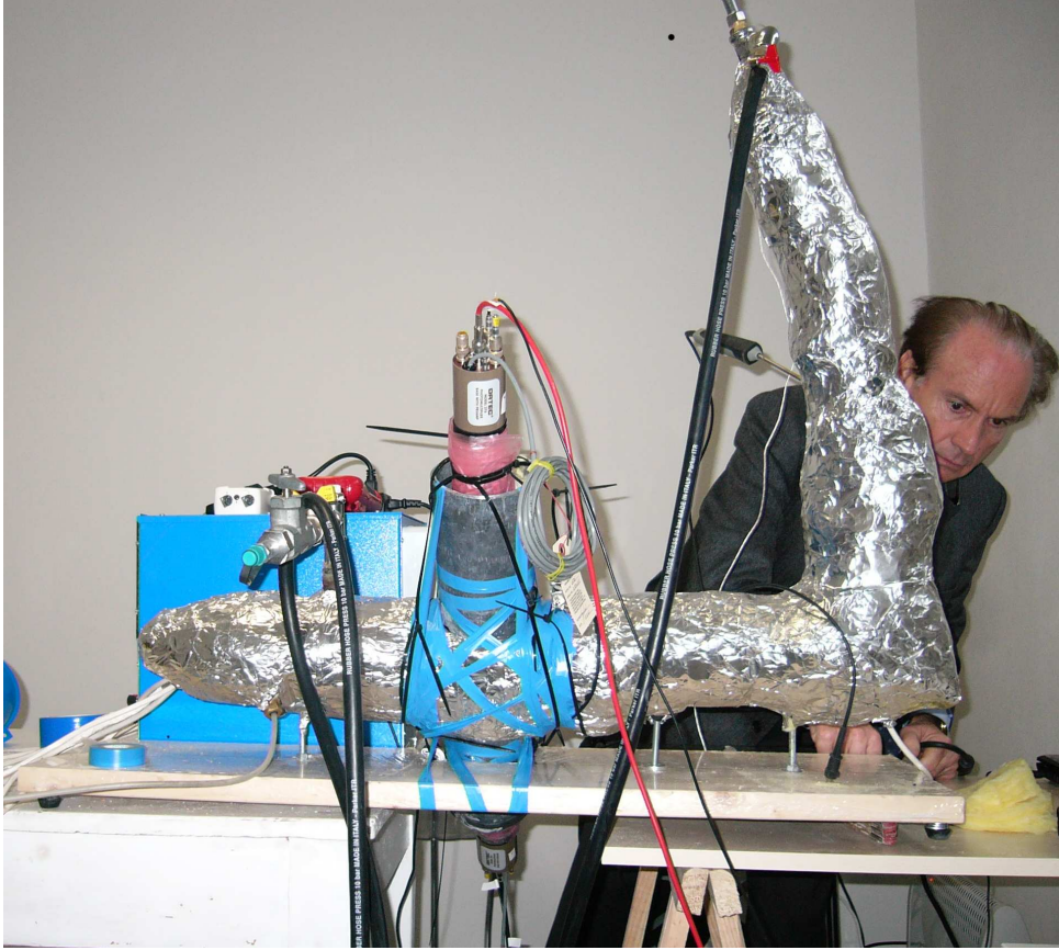
Figure 1: A photo of the apparatus. One scintillator detector is pointing upwards and is visible in the center of the picture, while the other is partially covered in the back.
