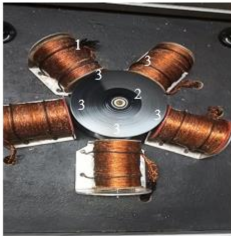
Figure 4. Design of a radiant charger using 5 coils and 5 poles of neodymium magnet.
